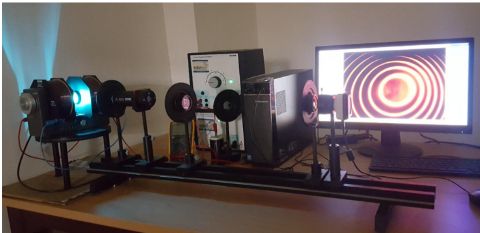
Figure 10.3: Zeeman Effect with Electromagnet
