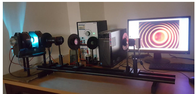
(c) Zeeman Effect with Electromagnet
